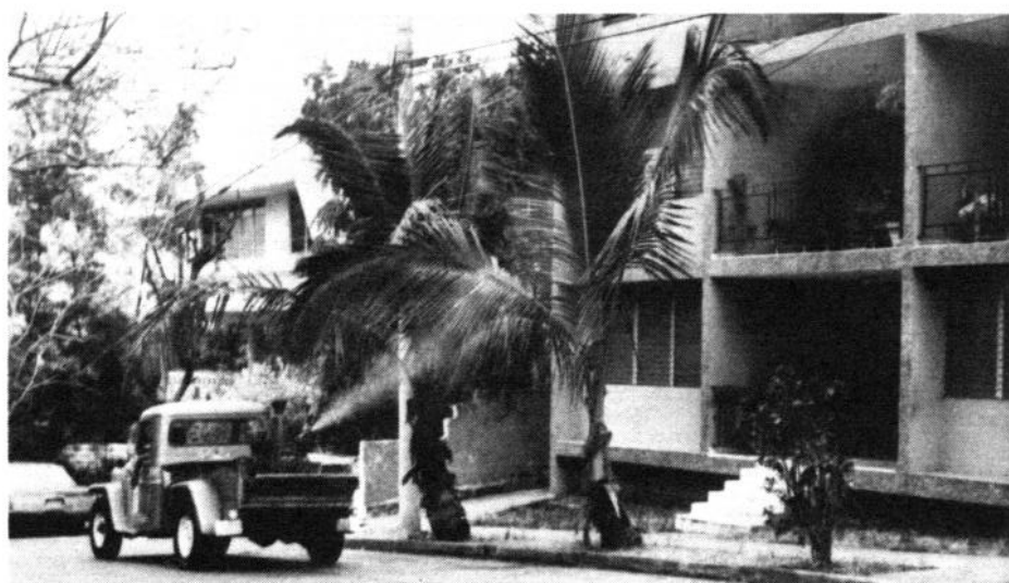
Application of insecticide in a residential area of Panama City to combat Aedes aegypti . The equipment being used is an ultra-low-volume cold aerosol generator mounted on a light truck.
